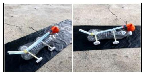
9. Test car by providing blowing air through balloon/straw launcher to create potential energy
