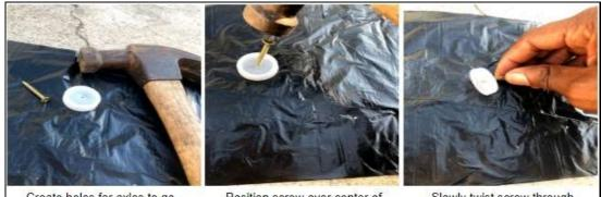
Create holes for axles to go through. Use a hammer and a 1/16" screw (Adult supervision required).
