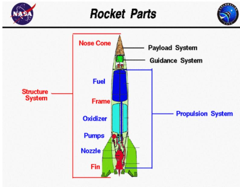
1. Structure system: this is the outer skeleton that includes all the parts that make up the frame of the rocket – the nose cone, frame, fins, and more. The material that the rocket is made from must be lightweight, but also strong.
