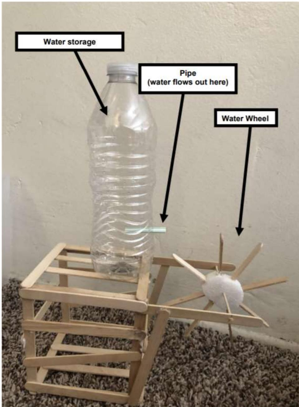
17. Testing your design. Grab a small container (no smaller than 6 inches wide x 6 inches long) and the water storage bottle, and fill up storage bottle at least halfway.
