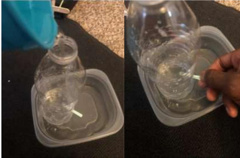
19. Position the water storage bottle on top of the structure with straw pipe directly over water wheel. Allow water to be released from the straw pipe. Allow water to collect in container below and re-use for further testing.
